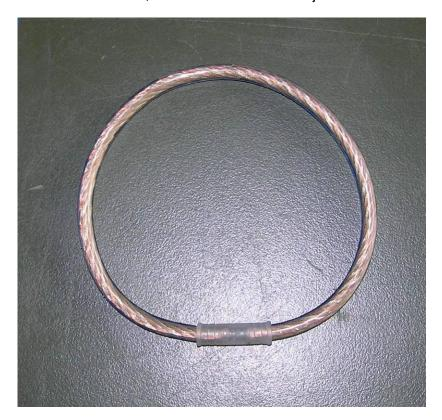
You insert the wire in the tube, keeping 10mm maxi between the extremities.
